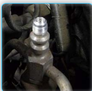
R12 access point
