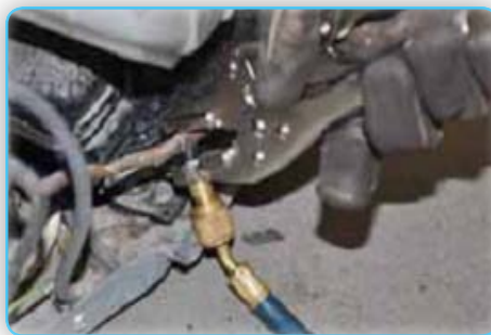
Piercing pliers connected to refrigerant line
