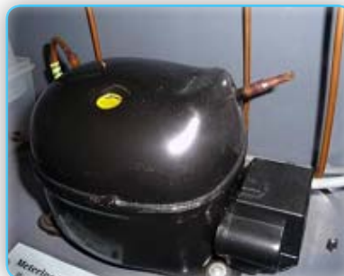
Process tube (crimped end)
