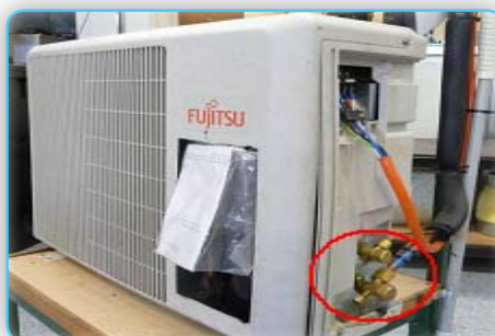
Split system air conditioner access ports
