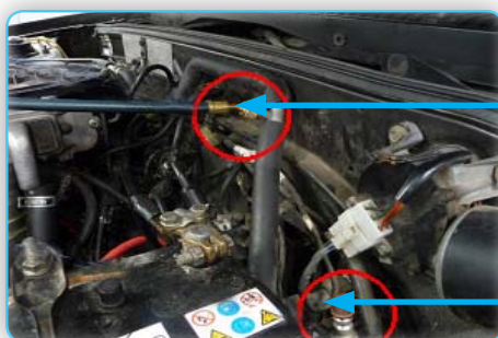
Vehicle air conditioner access ports
