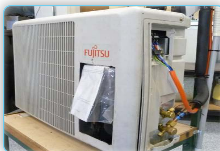
Split-system air-conditioner (external unit)
