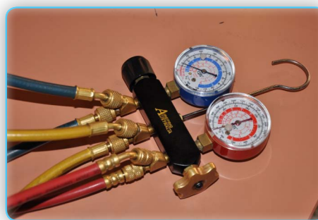
Service gauge manifold and service hoses with ball valves closed (left) and without ball valves (right)
