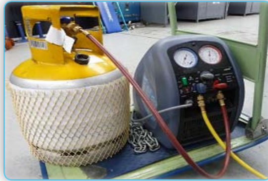
Recovery equipment set up on hand trolley
