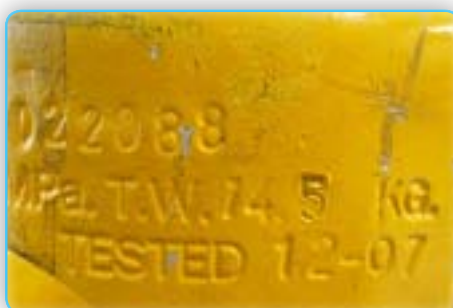
A test date stamped on the cylinder neck
