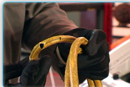
Refrigerant recovery unit with service hoses and connectors (left) and a deteriorated hose (right)
